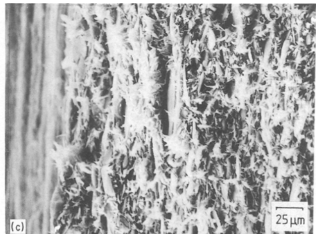
Figure 10 Scanning electron micrographs of the fracture surfaces observed close to the notch, after Instron testing at room temperature, for (a) PP/mica, 20%, (b) PP/mica, 40% and (c) PP/mica, 60%.
